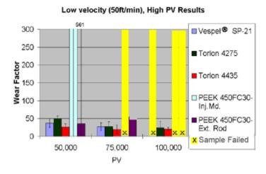
At medium velocity and medium pressure, Torlon 4435 showed a lower wear factor than Vespel ® and the PEEK sample failed altogether:
