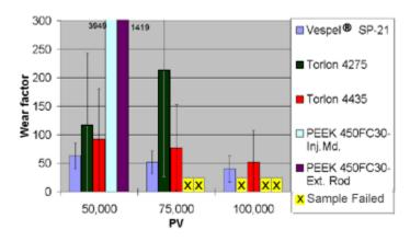
Although the wear performance of Vespel ® ran a close second to Torlon 4435 in most tests, Torlon 4435 is superior in cost efficiency, mechanical properties, and versatility.
