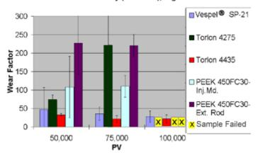
At high velocity and low pressure, the PEEK sample failed, while Torlon 4435 and Vespel ® showed good wear performance ratings:
